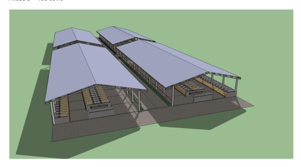
Internal, 9ft [2743] single rows and 16ft6inch [5092] head to head with 10ft [3048] scrape passage and 15ft6inch [4724] to feed barrier. 22ft [6706] between buildings.
