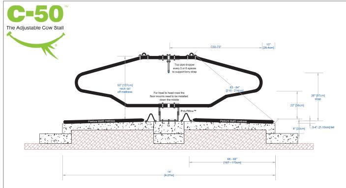
For fixing the floor mount bracket you need a minimum of 5inch [12.5cm] deep concrete pad
