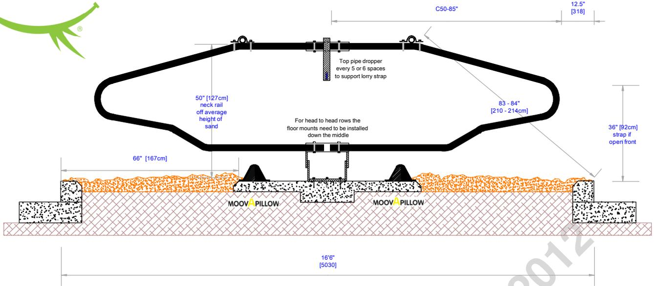
For fixing the floor mount bracket you need a minimum of 7inch [17cm] deep concrete pad
