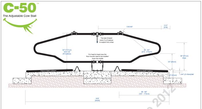
For fixing the floor mount bracket you need a minimum of 6inch [15.25cm] deep concrete pad
