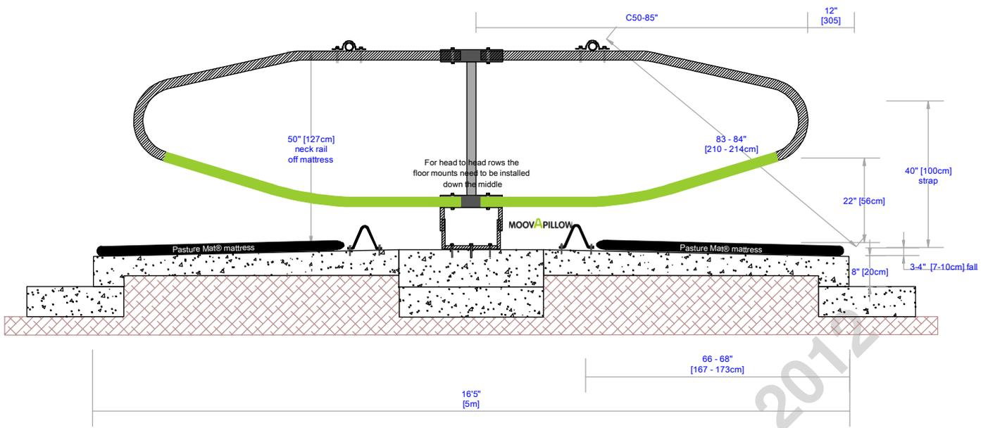
For fixing the floor mount bracket you need a minimum of 5inch [12.5cm] deep concrete pad
