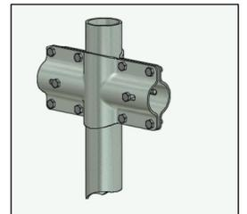
Note: Use the protective post sleeve and dent the post first to prevent it turning in the concrete
