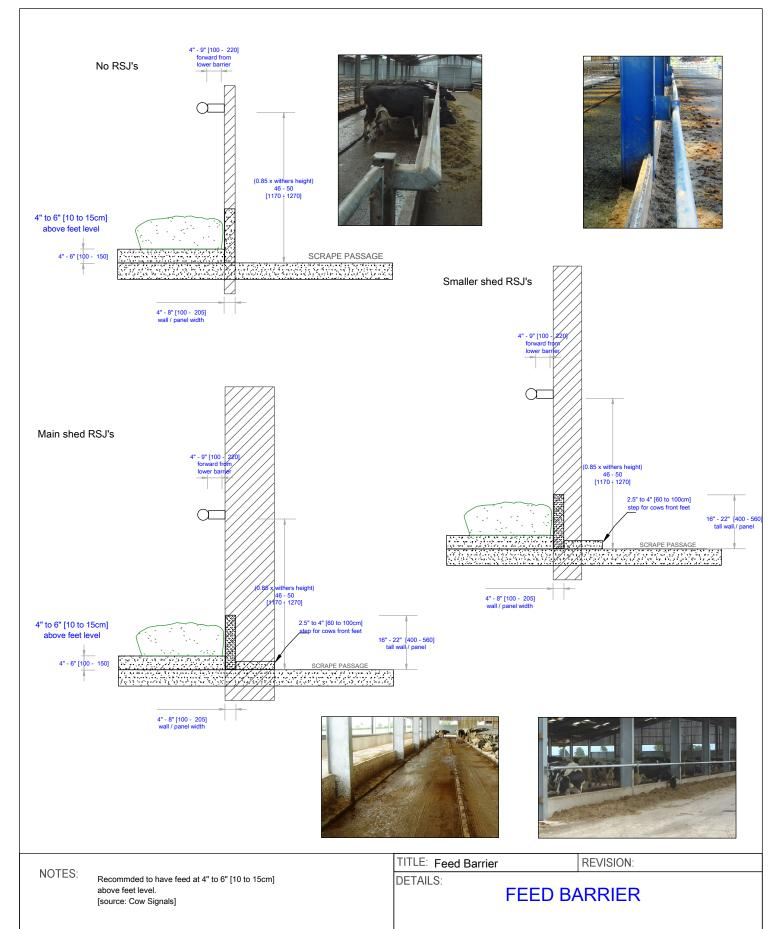
If front step is needed to guide scraper around steels, ensure it is a minimum of 14" wide step for front feet.
