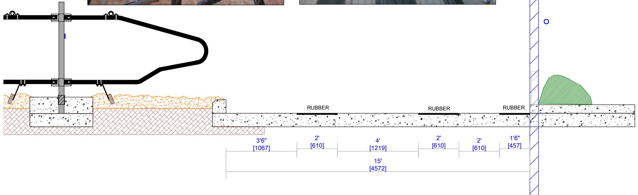
The rubber is 19 to 20mm thick
