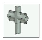
Note: Use the protective post sleeve and dent the post first to prevent it turning in the concrete
