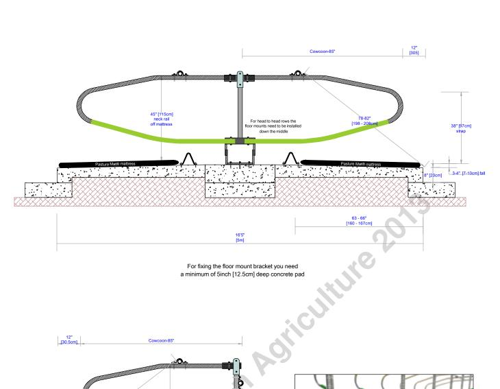
For fixing the floor mount bracket you need a minimum of 5inch [12.5cm] deep concrete pad
