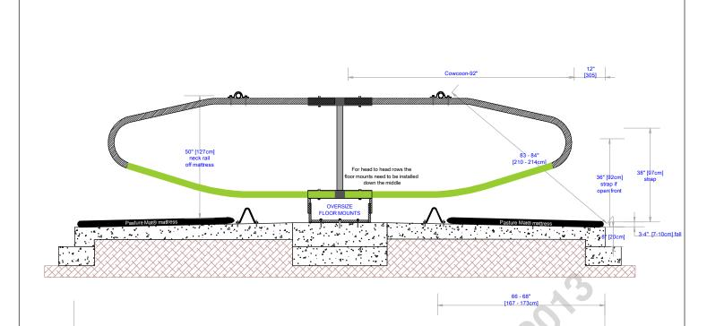
For fixing the floor mount bracket you need a minimum of 5inch [12.5cm] deep concrete pad
