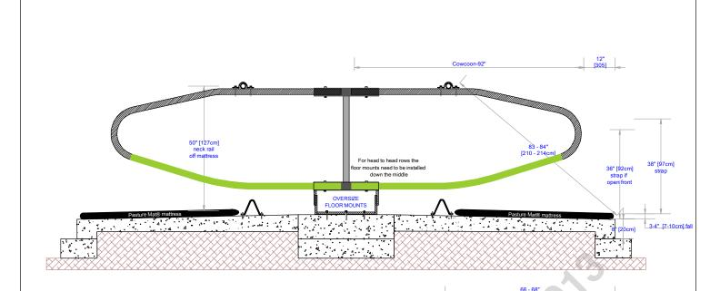
For fixing the floor mount bracket you need a minimum of 5inch [12.5cm] deep concrete pad
