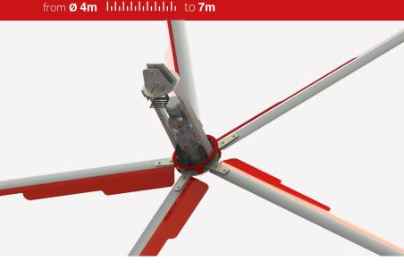
VS fans are axial destratifier with gear engine, extraordinarily functional and cost convenient. The particular feature of this series of products is the axial unloader, a patented component added to the mechanical part of the fans in order to eliminate the friction generated by the weight of the impeller and blades and increase their robustness. The VS fans are the traditional alternative to the ZEFIRO line and well suited for heavy-duty work situations.
