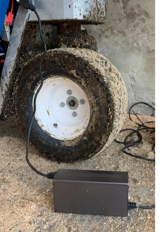
A battery charging protection pack protects the battery from voltage surges ensuring the BedMaid battery has a long lifespan.
