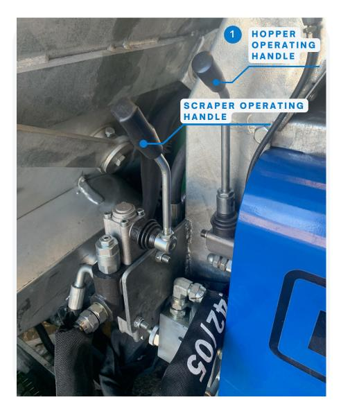
The hydraulic ram operates the tipping hopper saving the operator any heavy lifting
